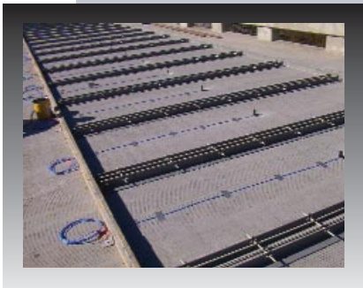
Figure 1 (above): Two 89 x 89 x 6-mm (3 1/2 x 3 1/2 x 1/4-in.) angle irons spaced about 1 m (3.5 ft) apart were embedded in each slab for electrodes in a back-to-back fashion. (IMG14730)
