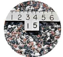
**Panel 15:** Three aggregates in three colors—dark green, white, and pink—are combined for another exposed aggregate surface. (IMG13745)
