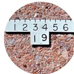
**Panel 19:** Pink feldspar aggregate makes a nice, somewhat sparkly pinkish-orange surface. This texture is very common for exposed aggregates. (IMG13749)
