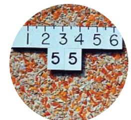
**Panel 55:** Special (non-reactive) orange glass and brown aggregate give a surface with excellent color retention. (IMG13775)
