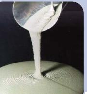
First use of ultra-high performance concrete for Sherbrooke pedestrian bridge in Quebec. Since then many projects have been built with ultra-high erformance concrete, also called reactive powder concrete, including a train station canopy in Calgary, Canada. (CT042)
