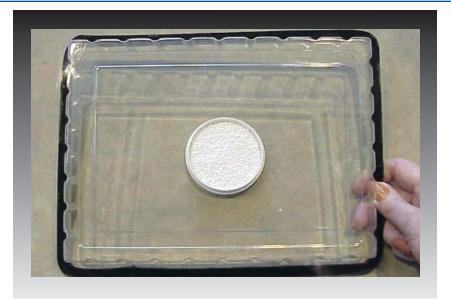
Moisture vapor emission rate is determined according to ASTM F 1869 using commercially available calcium chloride kits that absorb moisture from a specific test area over a known length of time. (IMG15989)
