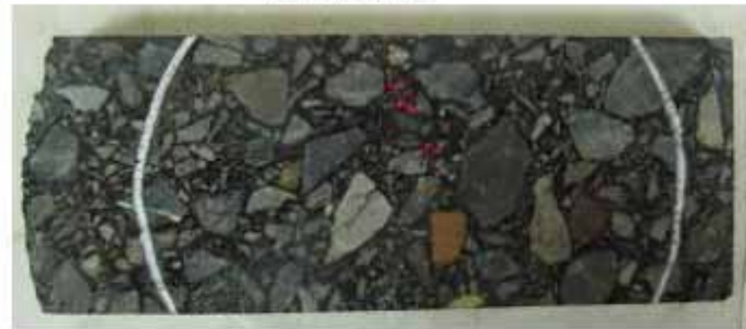
FIGURES 1 through 4 Initial steps in cutting gyrotory pill to obtain test specimens.
