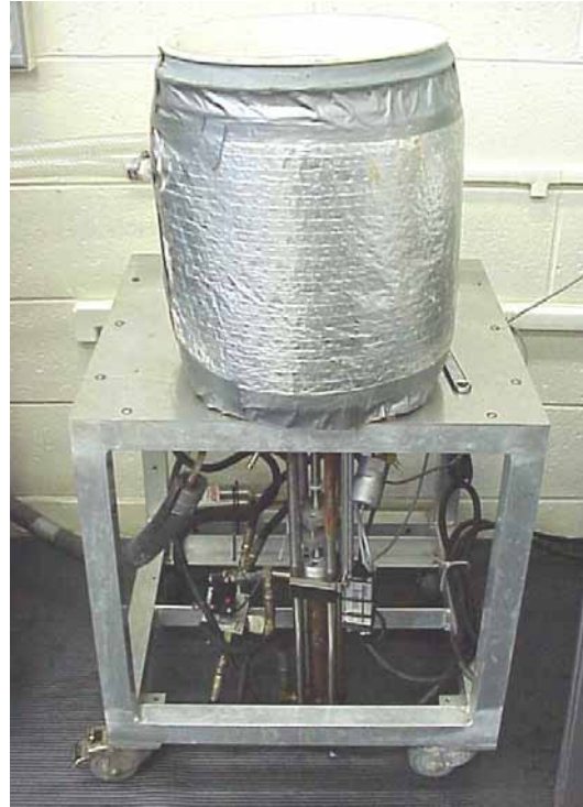
FIGURE 2 Portable test assembly: servohydraulic actuator (below) and temperature bath (above).
