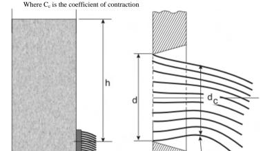
At the vena contracta, the volumetric flow rate Q of the fluid is given by  $\bullet$  Q = area of the jet at the vena contracta  $\cdot$  actual velocity =  $A_cV$
