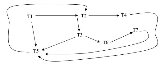
Since there is cycle in the wait- for graph  $(T_2 \rightarrow T_4 \rightarrow T_5 \rightarrow T_2)$  in the graph, therefore, system is in a deadlock.
