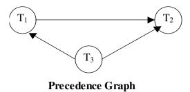
The given schedule is serializable. The serial orders of the transactions are:  $T_3$ ,  $T_1$ , and  $T_2$ .
