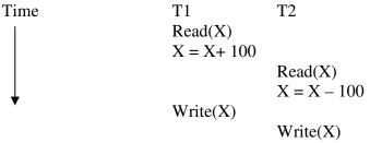
From the schedule, it can be seen that the updation of x by T1 will be overwritten by T2. If these transactions execute in serial order then the value of x should not change, but with this schedule the value of x will be reduced by 100, which is incorrect.
