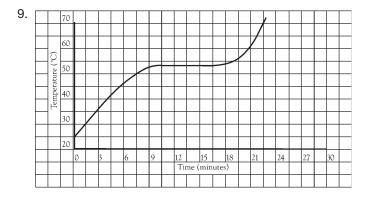
A sample of a pure solid substance is heated at a constant rate and its temperature recorded as a function of time. A graph of the data is shown above. At about what temperature is the heat added being used to melt the substance?
